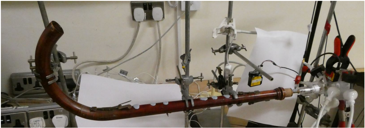
Figure 2. The mounting arrangement of the bass crumhorn, with six tone holes closed by BluTak. The laser displacement sensor is positioned above the upper key
