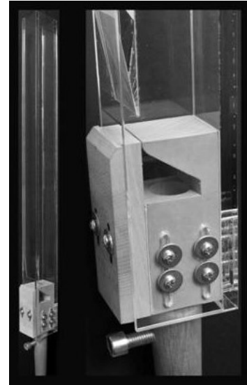
Figure 2. The adjustable experimental pipe with transparent walls
