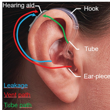
Figure 1: Behind-the-ear hearing aid, hook, tube and 3 typical feedback paths.
